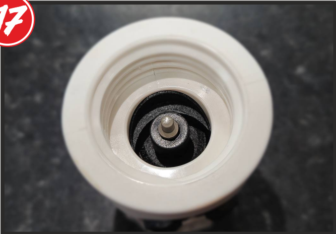
THE FIRING PIN CARRIER AND SLIDER SHOULD LOOK LIKE THIS IF THE SLIDER IS PUSHED ONTO SAFE. MAKE SURE YOU GET THE 'CRESCENT MOON' OF THE SLIDER FOR IT TO BE CORRECT.
