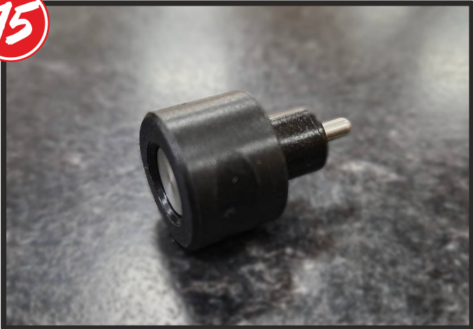
THE FIRING PIN AND WASHERS SHOULD BE PUSHED FULLY INTO THE FIRING PIN CARRIER. IT SHOULD NOT BE FLUSH.
