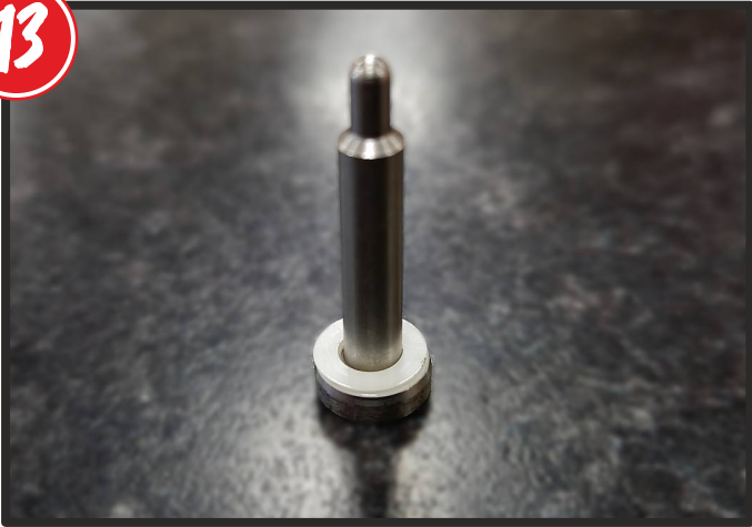
WASHERS ON THE FIRING PIN SHOULD LOOK LIKE THIS.
