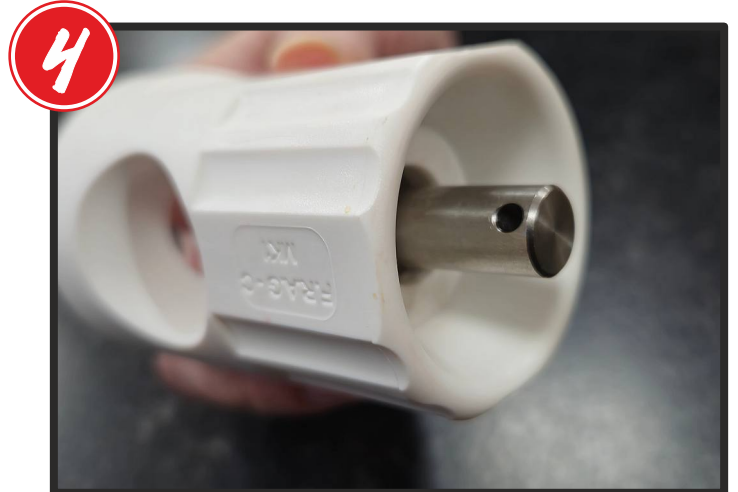
THE 3MM HOLE WILL BE VISIBLE AT THE TOP OF THE TRIGGER BAR.
