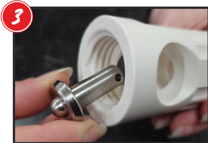
INSERT THE TRIGGER BAR (3) INTO THE MAIN BODY (5) UNTIL THE SHAFT WITH THE 3MM HOLE SHOWS AT THE TOP OF THE MAIN BODY.
