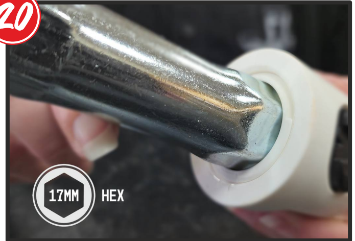
USE A 17MM HEX NUT TO TIGHTEN BOTTOM PLATE. WARNING! DO NOT OVER TIGHTEN THE BOTTOM PLATE.
