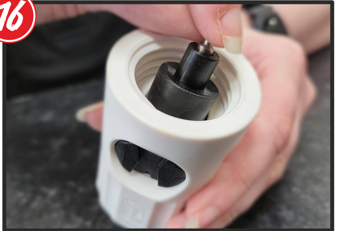
INSERT THE FIRING PIN CARRIER INTO THE MAIN BODY WITH THE PIN FACING UP TOWARDS THE BOTTOM OF THE FRAG. PUSH THE FIRING PIN CARRIER ALL THE WAY IN UNTIL IT TOUCHES THE TRIGGER BAR.
