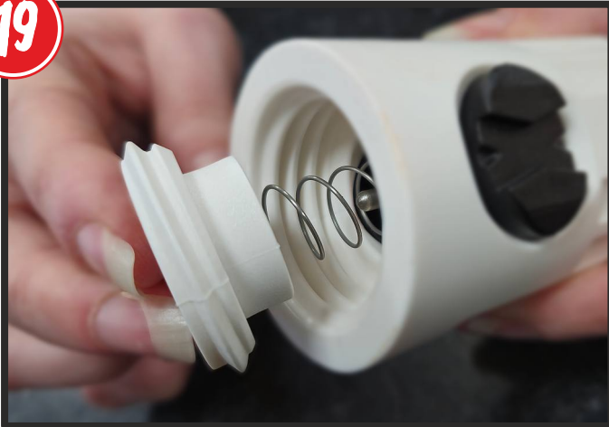
ADD THE BOTTOM PLATE (11) ONTO THE MAIN SPRING AND PUSH ONTO THE MAIN BODY AND SCREW DOWN CLOCKWISE WITH FINGERS.
