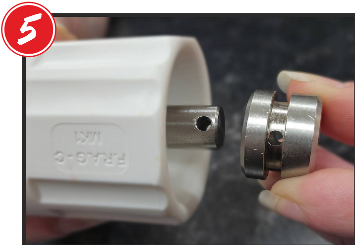
ATTACH THE TRIGGER WEIGHT (1) ONTO THE TRIGGER SHAFT (3) AND LINE UP THE HOLES FOR RETENTION PIN INSERTION.
