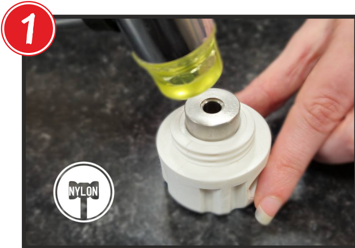
CAREFULLY HAMMER THE SSB INSERT (12) INTO THE SINGLE SHOT BASE (13) USING A NYLON HAMMER UNTIL IT IS FLUSH WITH THE BASE (SEE NEXT IMAGE).
